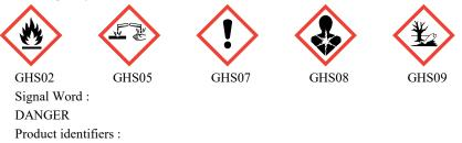
EC 918-668-5 HYDROCARBONS, C9, AROMATICS REACTION MASS OF ETHYLBENZENE AND XYLENE CAS 109159-24-2 RESINE POLYURETHANNE EC 200-751-6 BUTAN-1-OL
